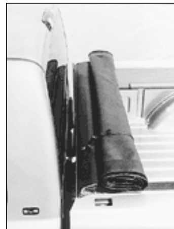
Cover rolled fully open with safety strap secured. NOTE: Cover is not rolled against cab to avoid wear on paint and cover.
